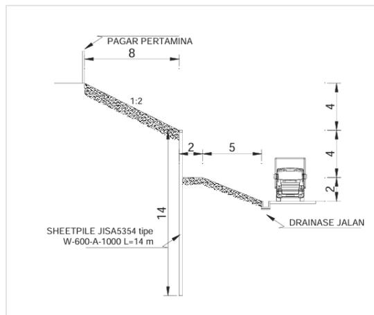
Fig. 3 Slope model and sheet pile structure
