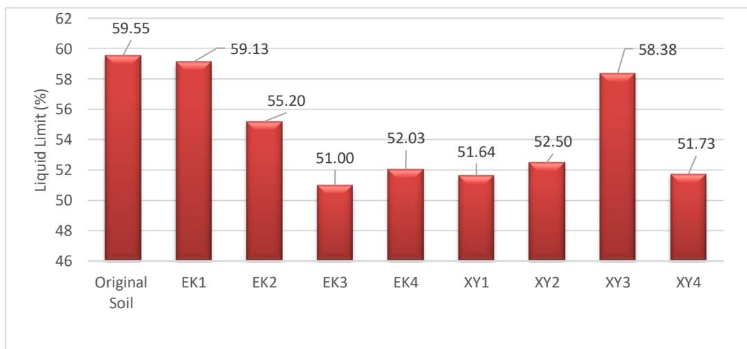
Fig. 3 Liquid limit of clay soil
