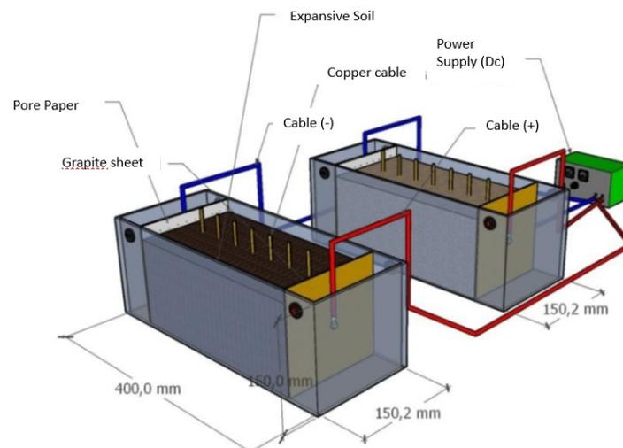
Fig. 3 Electrokinetic improvement: apparatus for electrokinetic clay improvement
