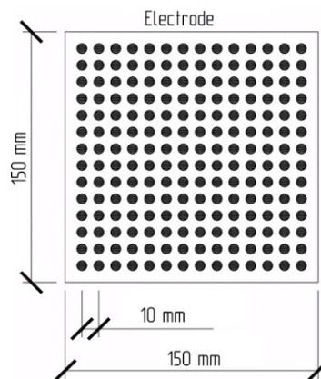
Fig. 2. Electrokinetic improvement: electrode
