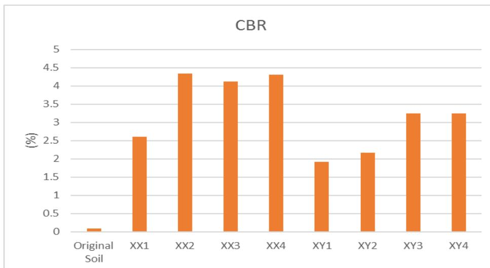
Fig. 5 CBR value of electrokinetic improvement
