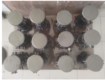
Fig. 5 Concrete molding process
