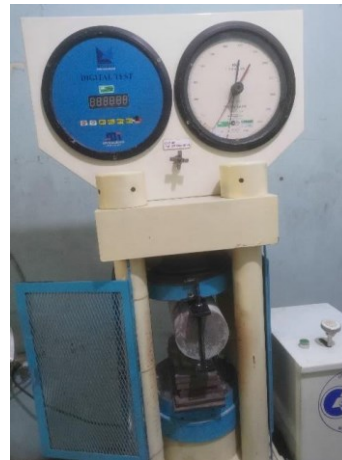
Fig. 8 Split tensile strength test
