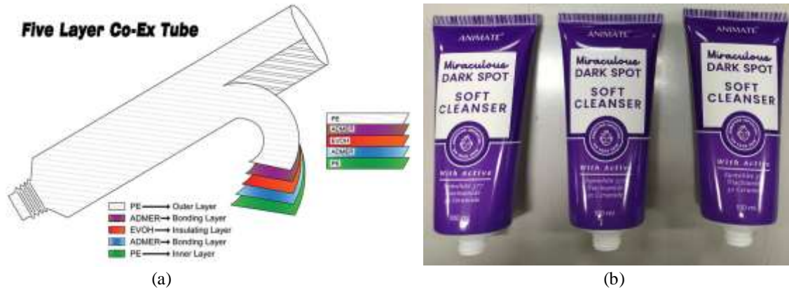
Figure 1. An example of co-extruded tubes; (a) Layer cross-section; (b) Final products after printing
