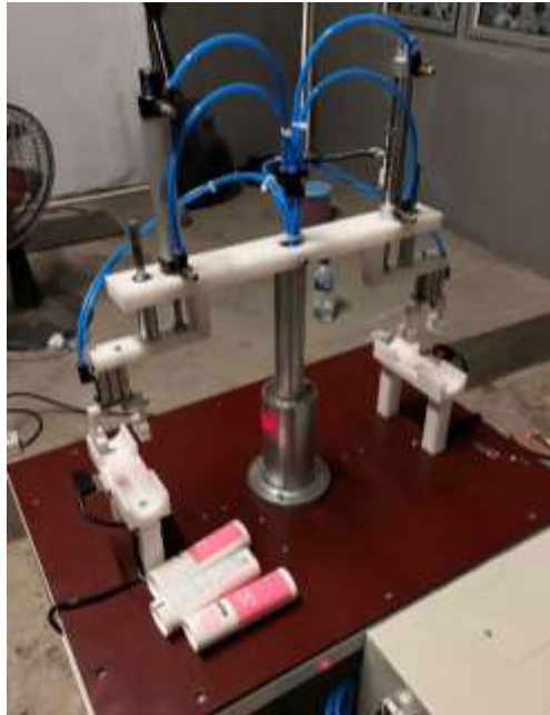
Figure 13. The realization of the swivel arm unit and the gripper unit with a lifting mechanism
