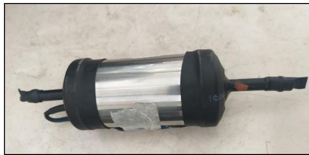
Figure 2: Electromagnetic-based fuel-saving device.
