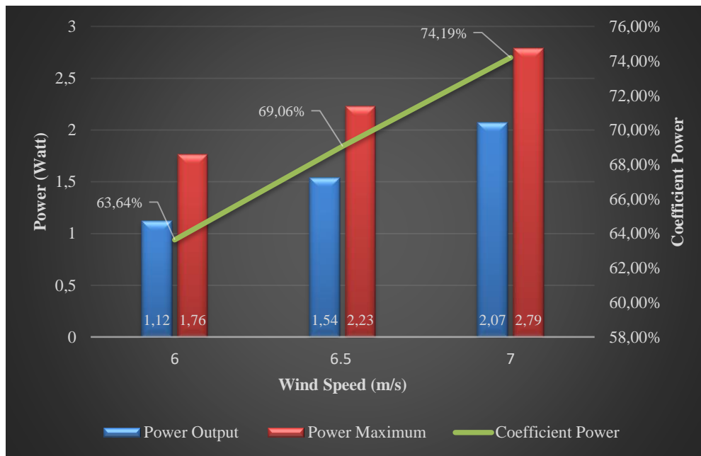
Figure 2. Comparison Graph of Maximum Power Value to Power Output
