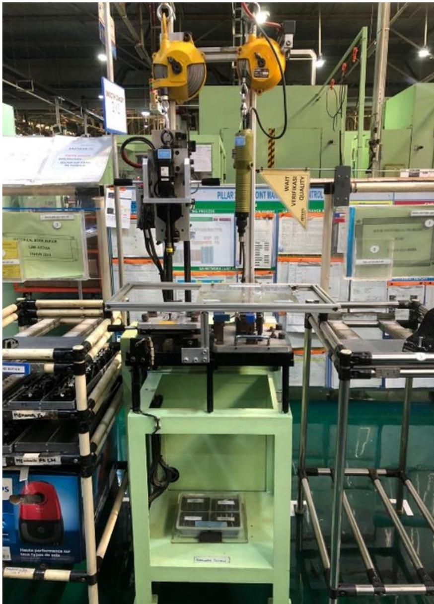
**Gambar 8. Aktual Mesin *Install screw Contingency Door lock***
