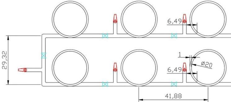
Fig 3. Flocculator prototype design, tank 1-6 from right below to right above (Front View)
