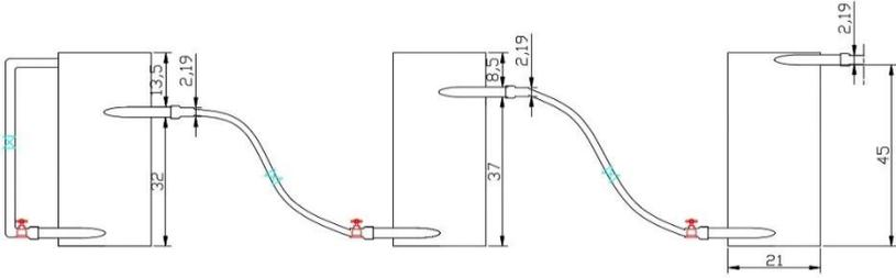
Fig 2. Flocculator prototype design, tank 1-3 from right to left (Side view)
