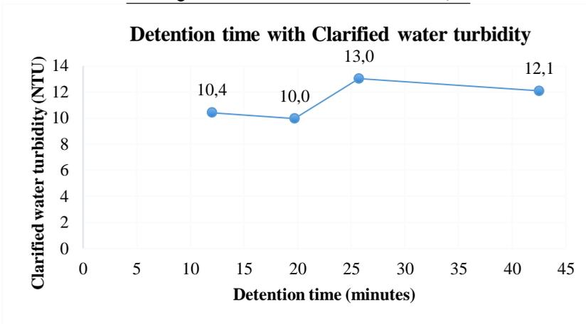
Fig 6. Detention time effects to clarified water turbidity
