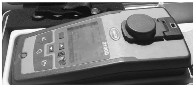
**Fig 5.** Turbidimeter that used in research
