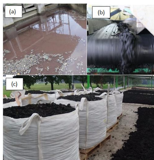
Figure 1. (a) The Industrial Wastewater ; (b) Mechanical separation of solid particles from wastewater; (c) Dried sludge
