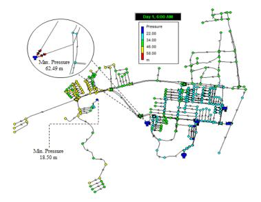
Fig. 9. The simulation results of the pressure on each node during peak hours
