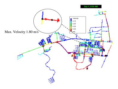
Fig. 10. The simulation results of velocity in each pipe during peak hours
