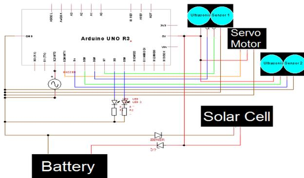
Figure 4. Arduino Connection
