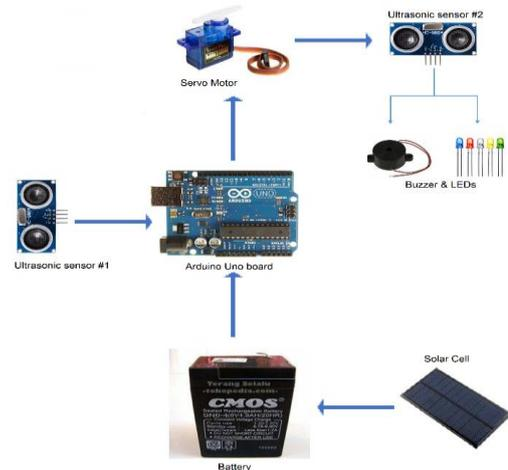
Figure 2. Block Diagram of Smart Trash Bin with Solar Cell
