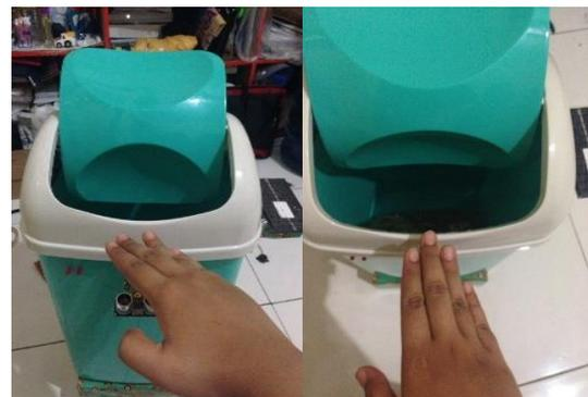
**Figure 6.** Ultrasonic sensor #1 detect an object & the automatic lid opened
