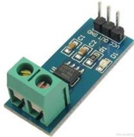
**Figure 4. ACS-712 current sensor module**
