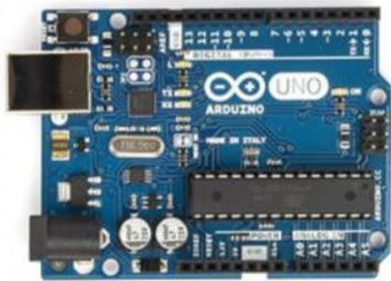
Figure 1. Arduino UNO R3 Microcontroller
