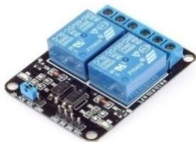
Figure 10. Two-channel relay module
