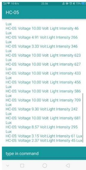
**Figure 8. The reading of HC-05 Bluetooth module**
