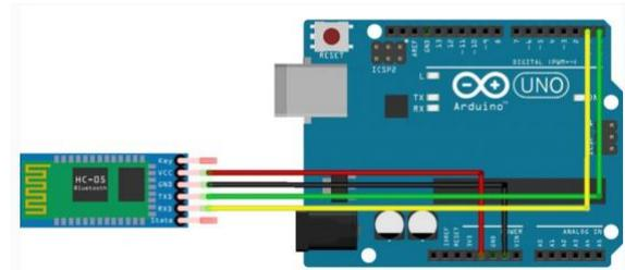
Figure 4. Arduino Uno to HC-05 Bluetooth module
