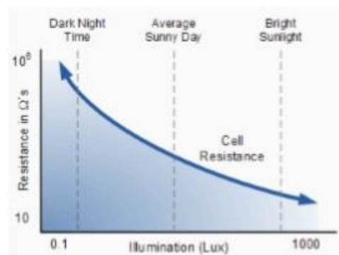
Figure 6. The resistance vs illumination graph of LDR
