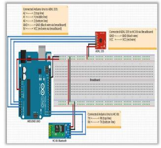
Fig. 2. Arduino circuit design
