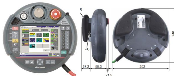
Gambar 2. Teaching Pendant R56TB dan Enable Switch Sumber : Melfa. 2013. Mitsubishi Industrial Robot R56TB Instruction Manual
