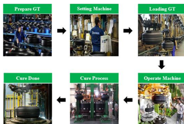
Gambar 5. Diagram Alir Proses Cure Ban
