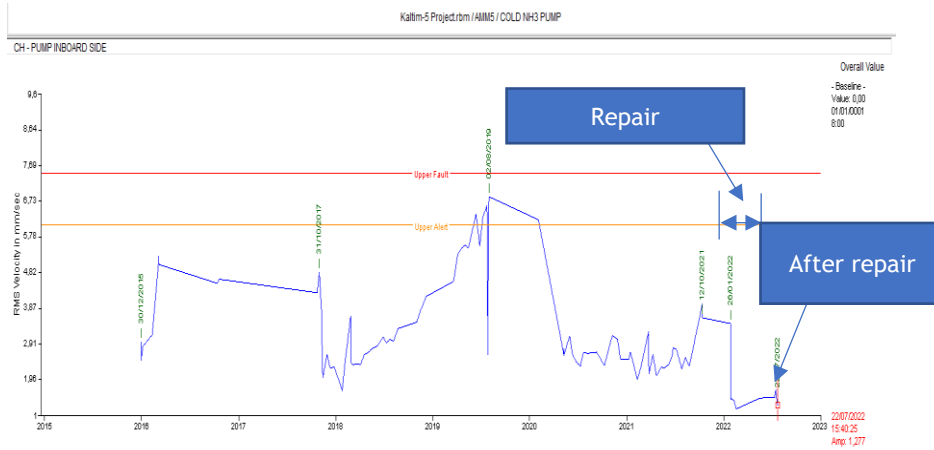
Figure 9. Vibration trend Pump 110-J after repair.
