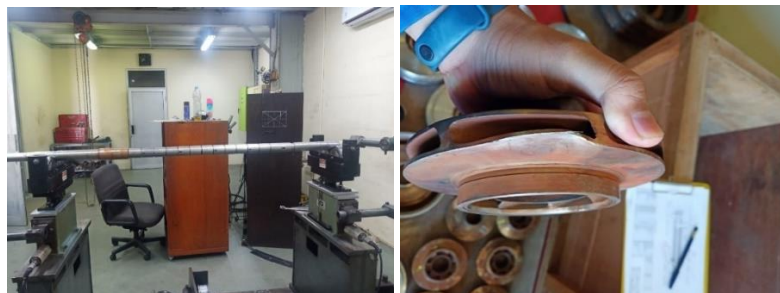
Figure 6. Pump shaft was bending and the wearing ring and impeller were rubbing
