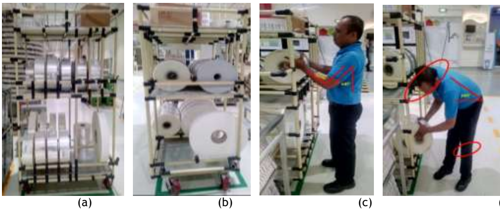
Figure 2. (a) front view of current materials pallet; (b) side view of current materials pallet; (c) working methods from middle side of materials pallet; (d) working methods from bottom side of materials pallet
