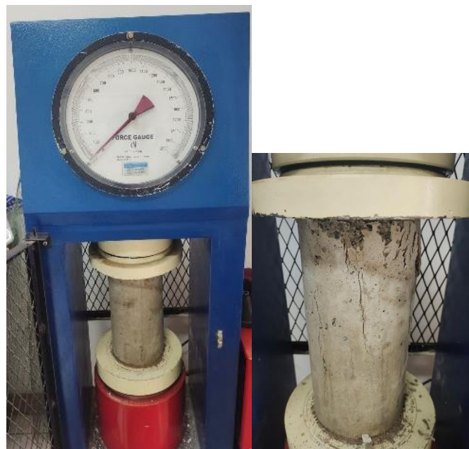
Fig. 7 Compressive strength test and a tested specimen
