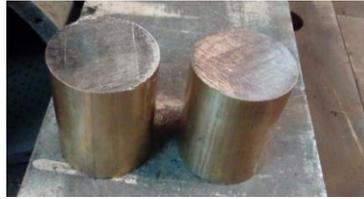
Gambar 14. Material piston pompa
