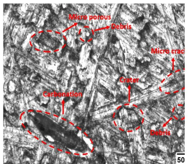
**Fig 9. Surface Morphology of Samples Using Microstructure With Variation of Peak Current (a) 8A, (b) 10A, (c) 12A**
