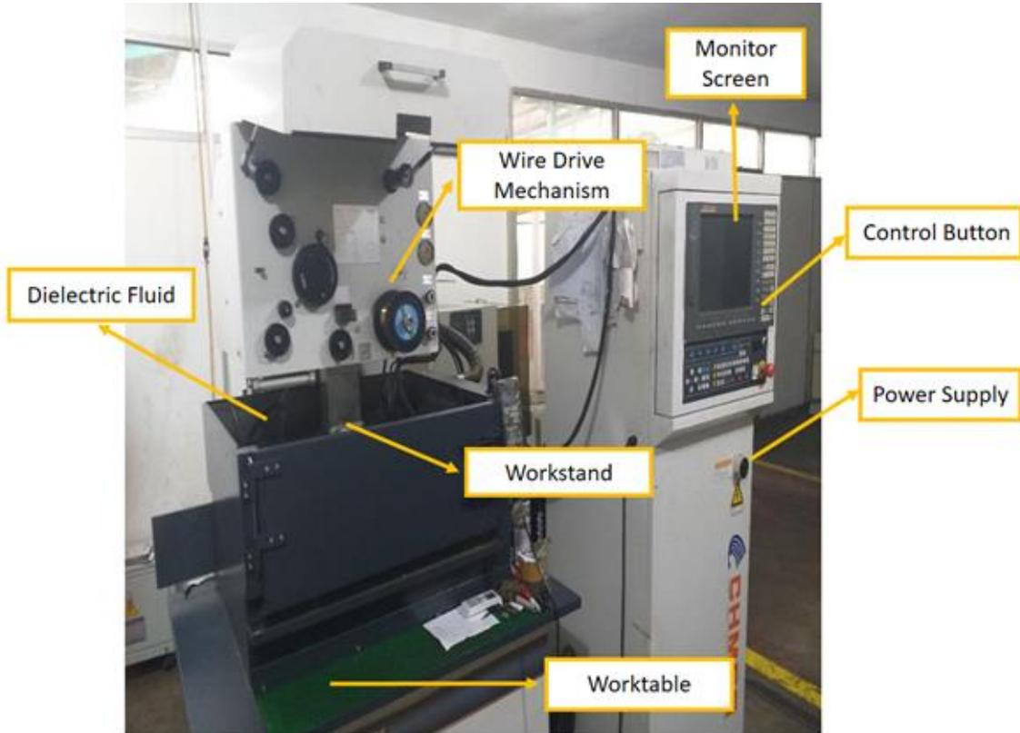
**Fig 1. Wire-cut Chmer type GX 360 L**
