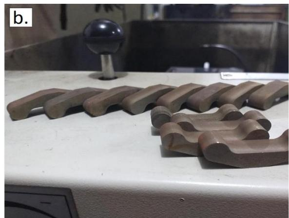
**Fig 11. WEDM Process Results a. Cut Workpiece, b. Chain Component Results**
