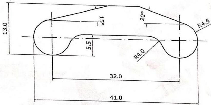
**Fig 3. Workpiece Job Sheet Chain Components**
