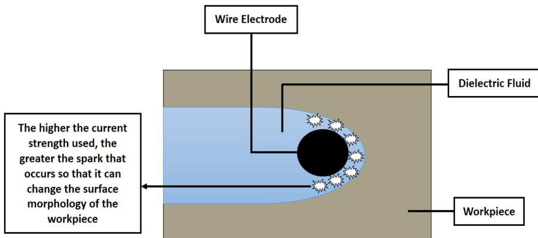
**Fig 10. Illustration of Cutting in the WEDM Process**
