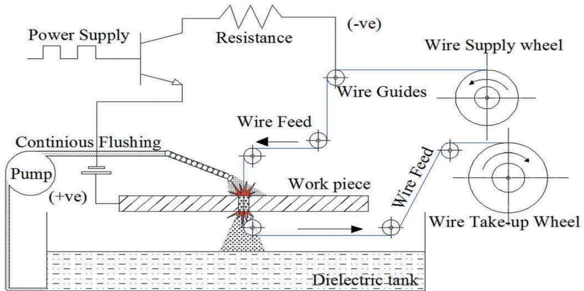
**Fig 8. Principle of WEDM Process [20]**
