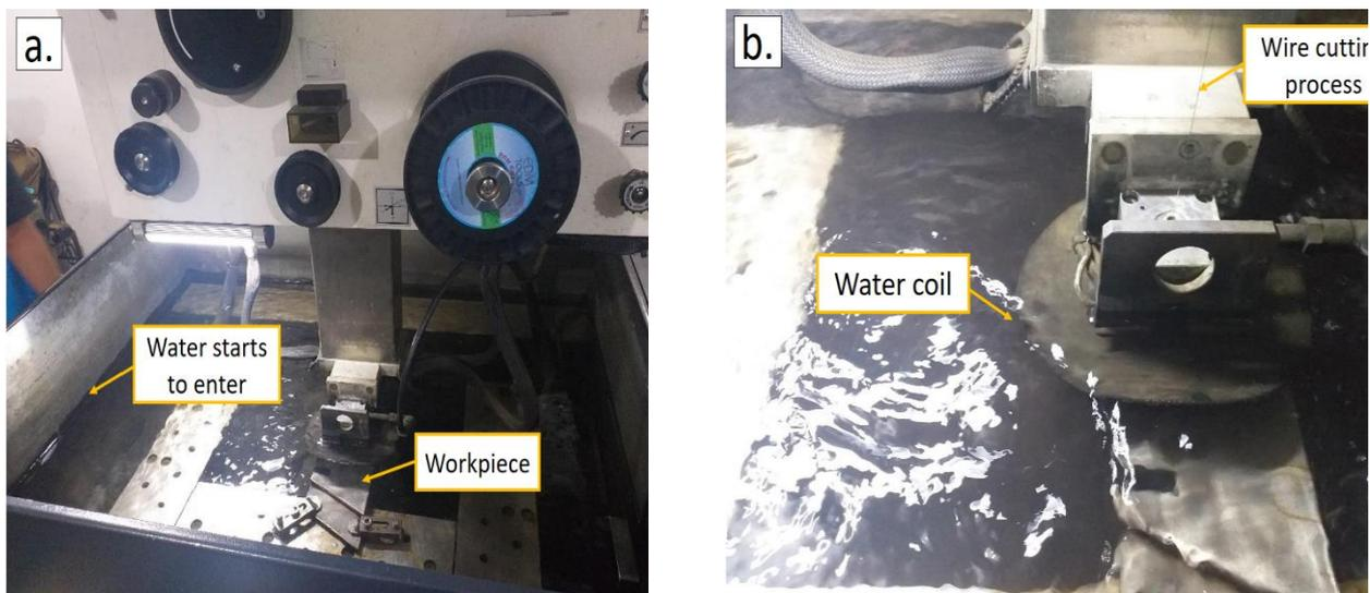
**Fig 7. Process of Running Program Matching Process a. Dielectric Fluid Begins to Enter the Work Area, b. Workpiece Cutting Process**
