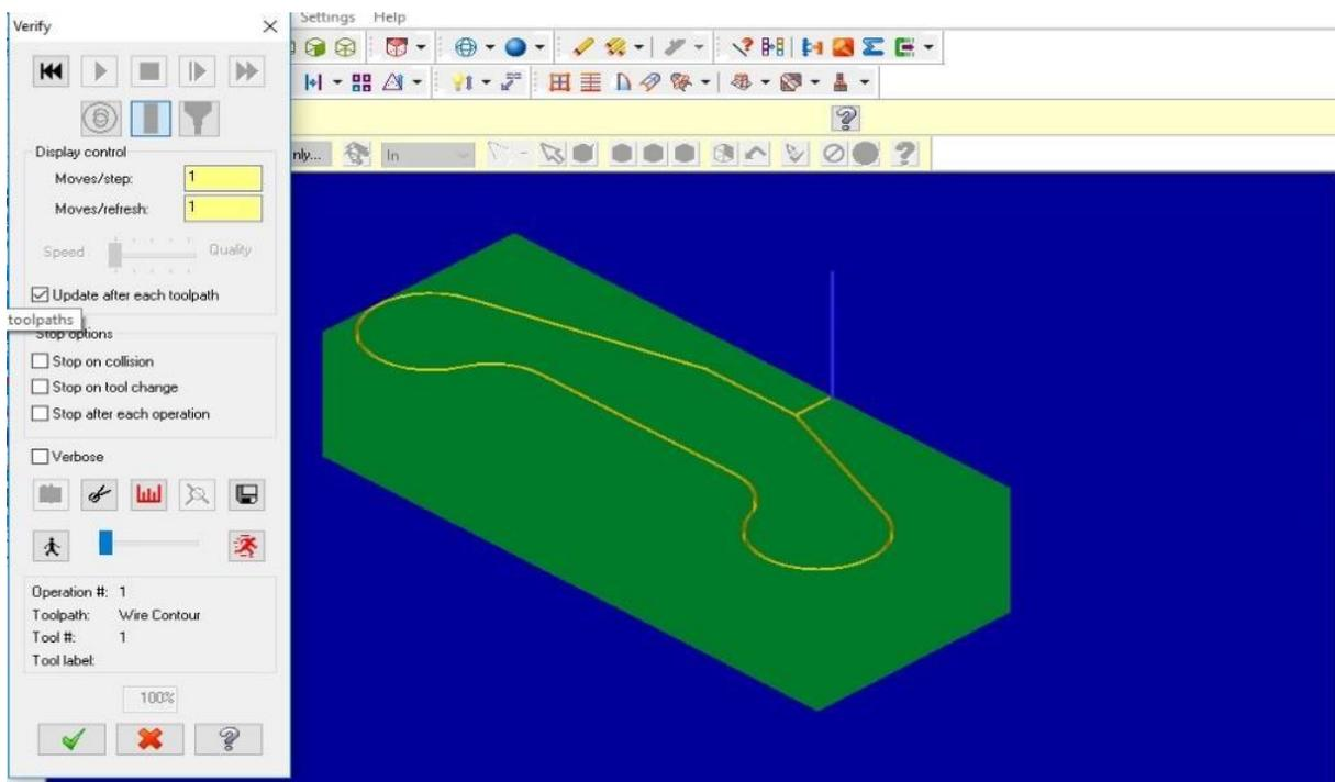
**Fig 6. Simulation of the Chain Component Manufacturing Program**
