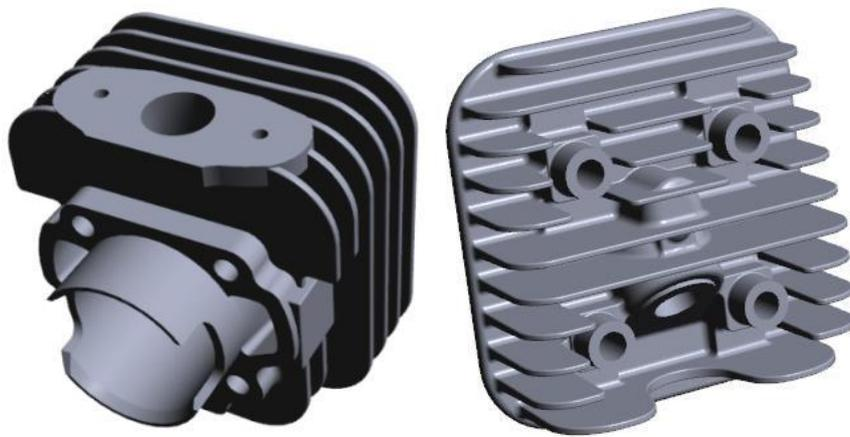
Gambar 10. 3D *solid* blok silinder & *comp. head*.
