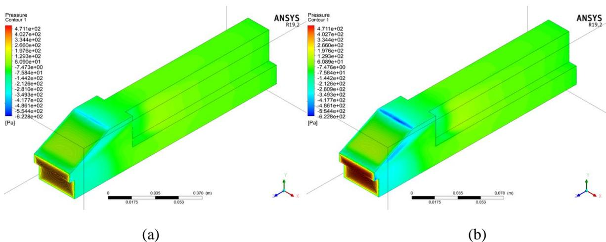
**Fig. 7** Pressure Contour in locomotive body in the wind velocity (a) 25 m/s, and (b) 29 m/s. Seen, the pressure is increasing as the velocity increase.
