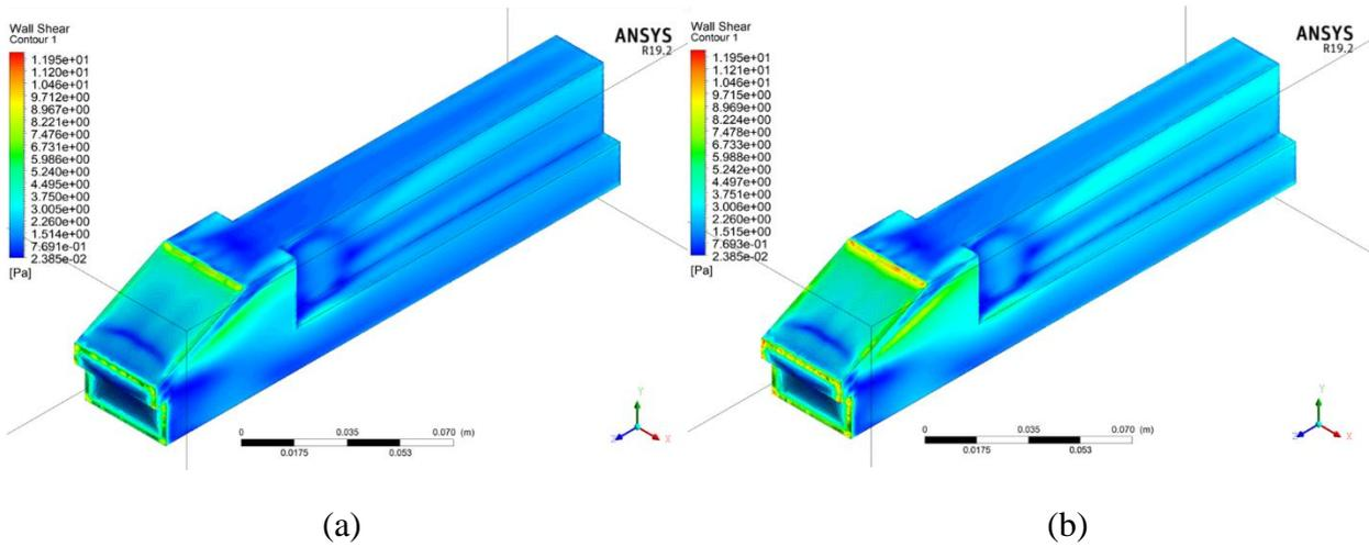
**Fig. 8** Shear Stress Contour in locomotive body in the wind velocity (a) 25 m/s, and (b) 29 m/s. Seen, the shear stress is increasing as the velocity increase.
