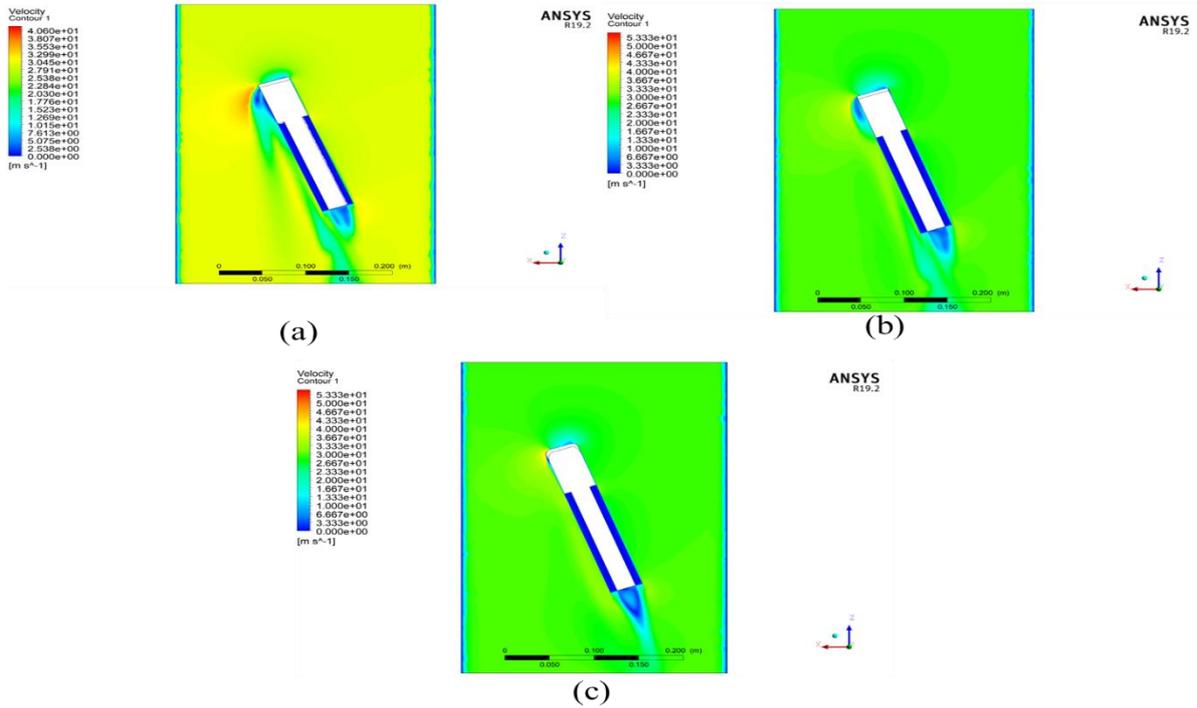
**Fig. 17** Velocity Contour around the locomotive at  $20^0$  yaw angle in the Geometry Options (a) CC203; (b) 1; and (c) 2 at velocity 29 m/s. Seen, the turbulence of the flow is decreased as the design change.
