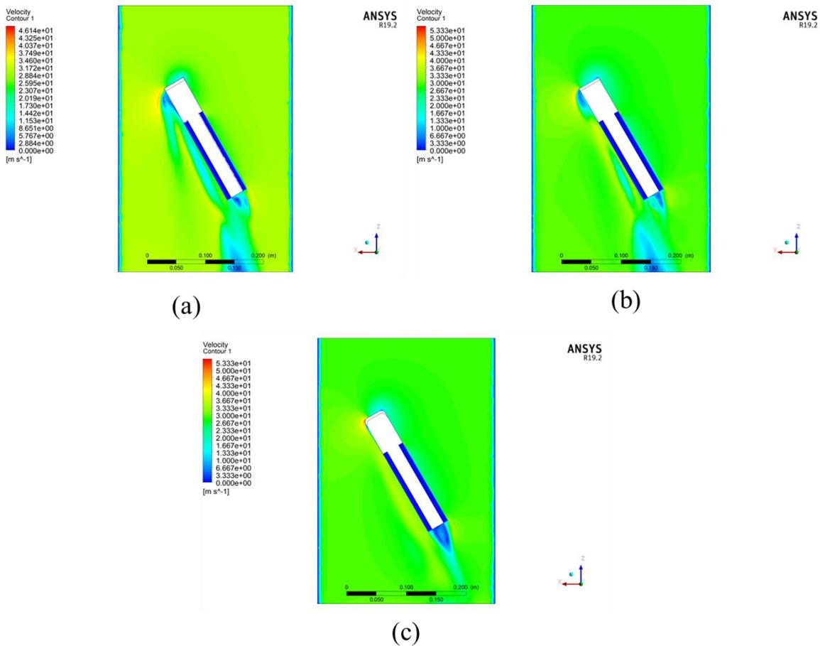
**Fig. 18** Velocity Contour around the locomotive at  $30^0$  yaw angle in the Geometry Options (a) CC203; (b) 1; and (c) 2 at velocity 29 m/s. Seen, the turbulence of the flow is decreased as the design change.
