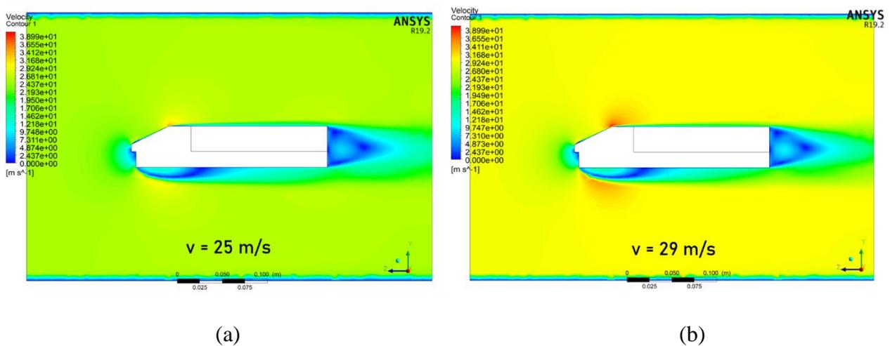
Fig. 6 Velocity Contour around the locomotive in the wind velocity (a) 25 m/s, and (b) 29 m/s. Seen, the turbulence of the flow is concentrated at the corners of the muzzle of the locomotive, and the turbulence is increasing as the velocity increases.
