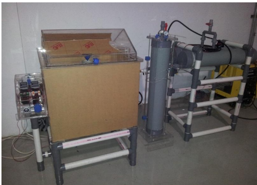
Gambar 2. Rancangan Salt Spray Test Chamber
