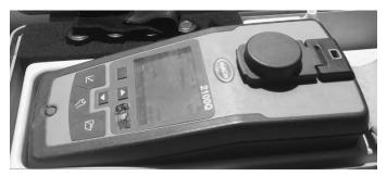
Fig 5. Turbidimeter that used in research
