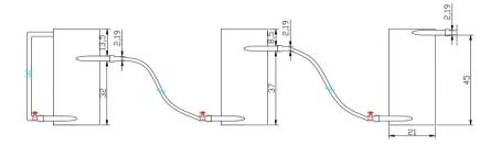
Fig 2. Flocculator prototype design, tank 1-3 from right to left (Side view)
