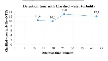
Fig 6. Detention time effects to clarified water turbidity
