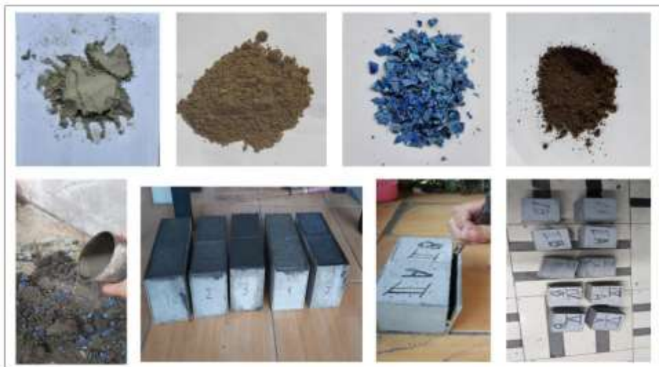
Fig 3. Paving Block Making Process
