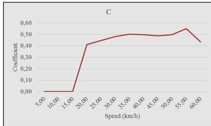
Fig. 12. Relation between coefficient of effectivity vs wind speed.
