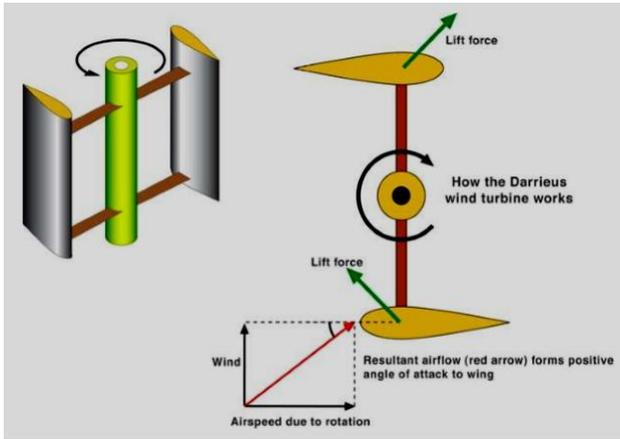
Fig. 2. Working principles of a lift-type vertical axis wind turbine (VAWT) [OH05].
