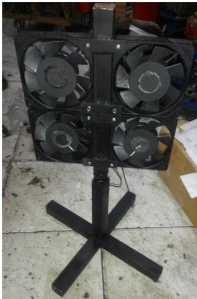
Fig. 7. The tower consisted of four PC fans with multiblades.
