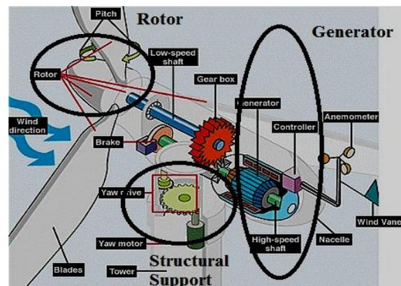
Fig. 1. A general pattern of a horizontal-axis wind turbine (HAWT) which emphasizing its three main parts: rotor, generator, and structural support [WT].
