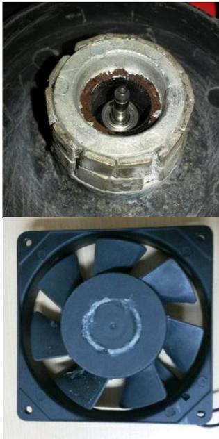
Fig. 6. Placing magnet on the iron surface (left) and the finished PC fan (right).
