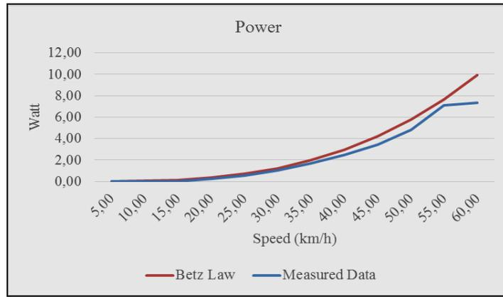
Fig. 13. Relation between output power vs wind speed.
