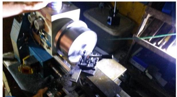
Fig. 3. The middle of the fan that close to the iron is cut with lathe machine.
