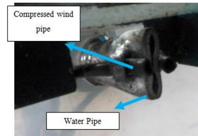
Fig.10. Water and Wind Output
