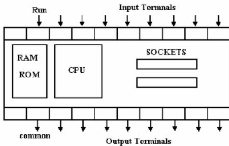
Fig 7. PLC Diagram [DJD14].
