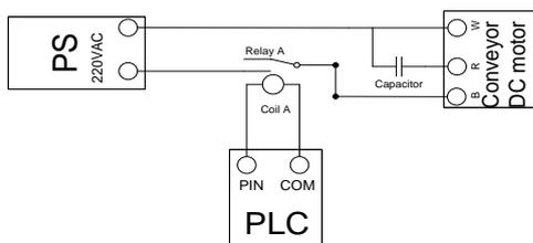
Fig. 16. Induction Motor Circuit Diagram [RCN14]
