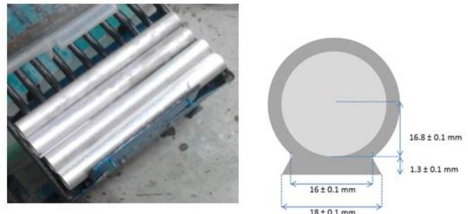
Fig.1. Modulator and its Dimension
