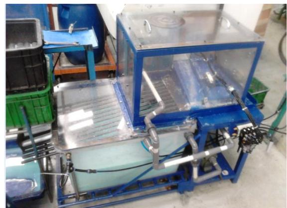
Fig.2. Automated Modulator Washing Device
