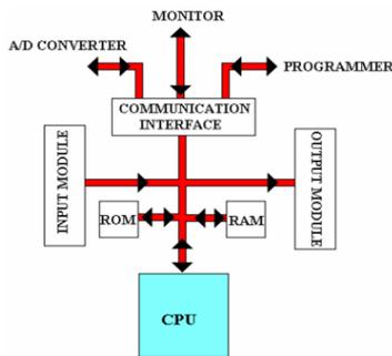
Fig.8. Oversimplified PLC Diagram [DJD14]
