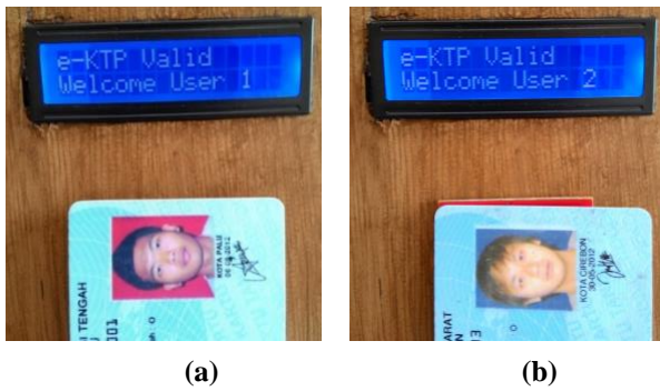
Figure 17. Display When Authorized e-KTPs are read; (a) User 1 (Mode 1), (b) User 2 (Mode 2)
