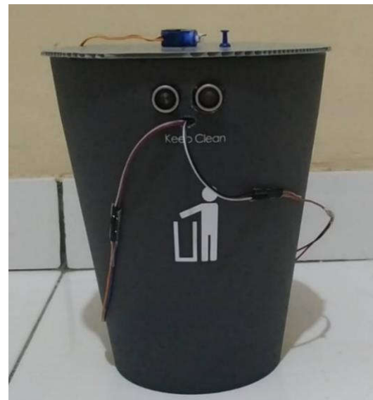
Figure 5. Appearance of Smart Dustbin Prototype. The two eyes-like protrusion is the ultrasonic sensor to detect user's hand.
