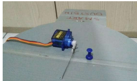
Figure 4. Placement of Servo motor on the lid. To open and close the lid, the servo is connected to the moving lid using a string.
