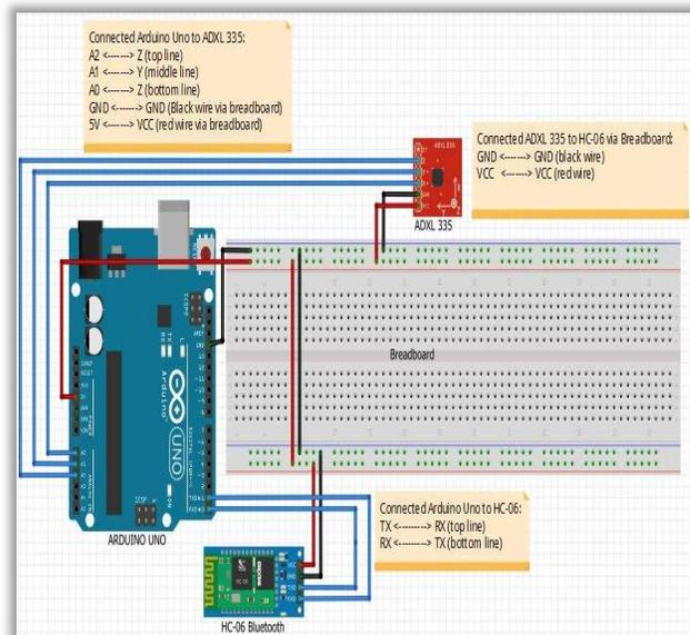
Fig. 2. Arduino circuit design
