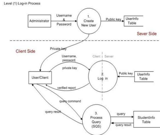
Figure 3.2. XMLDsig based SQS level (1) Log-in Process
