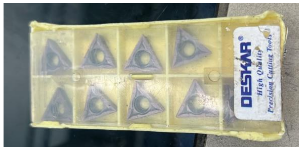
Figure 3. TCMT16T304 Inserted Carbide Cutting Tool.
