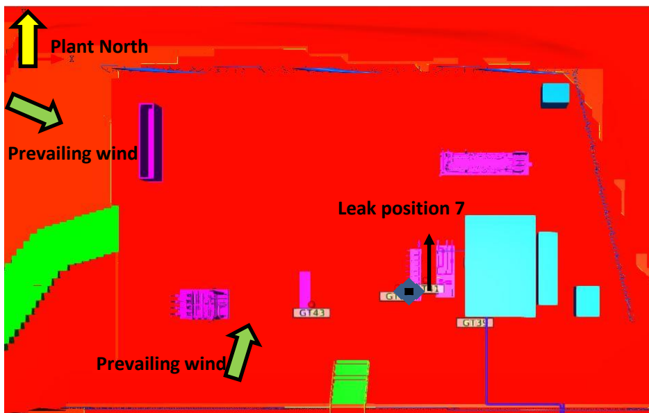
Figure 5 Leak position and leak direction in Area 3 for CO 2 dispersion simulation
