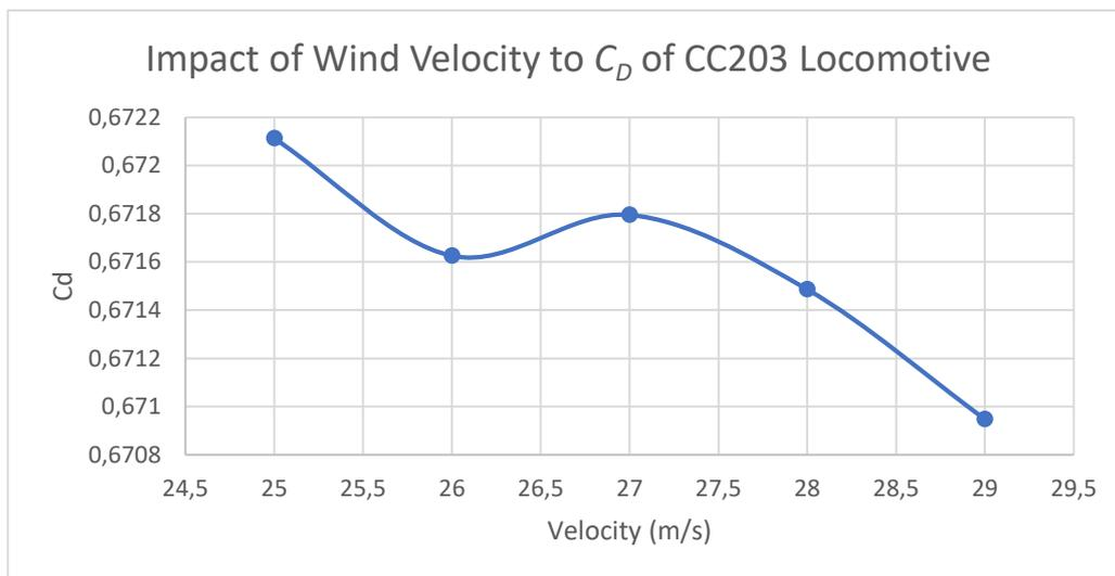
**Fig. 4** Graph of Changes in Wind Velocity against  $C_D$  Value of CC203 Locomotive
