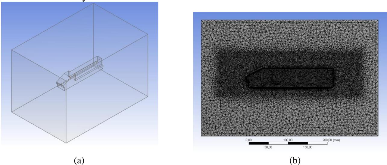
Fig. 2 (a) Modelling and enclosure used in this research; (b) Meshing
