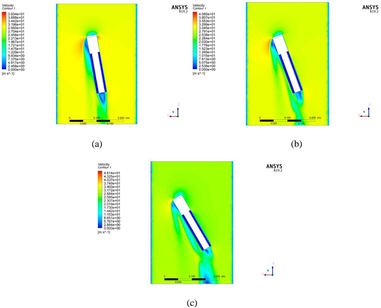
**Fig. 9** Velocity contour of yaw angle: (a)  $10^0$ , (b)  $20^0$ , dan (c)  $30^0$
