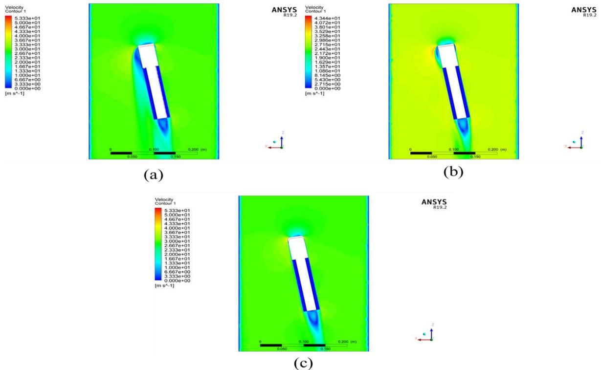
**Fig. 16** Velocity Contour around the locomotive at  $10^0$  yaw angle in the Geometry Options (a) CC203; (b) 1; and (c) 2 at velocity 29 m/s. Seen, the turbulence of the flow is decreased as the design change.
