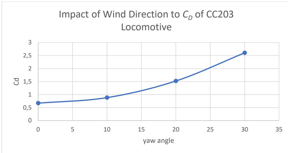
Fig. 5 Graph of Changes in Wind Direction against  $C_D$  Value of CC203 Locomotive
