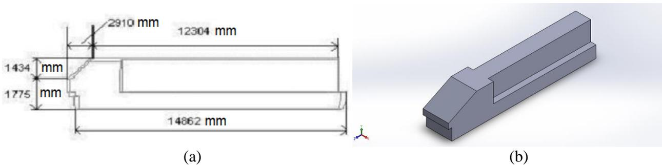
Fig. 1. (a) Dimension of CC203 locomotive [2]; (b) Modelling of CC203 locomotive
