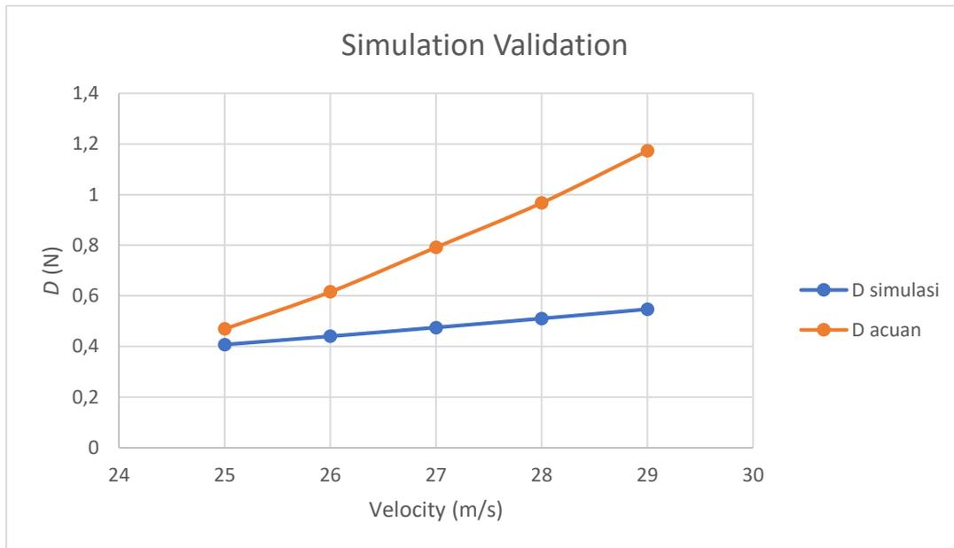
**Fig. 3** Simulation Validation Graph. The “D simulasi“ is for CFD simulation results, and “D acuan“ is for Wulandari’s research results [2]
