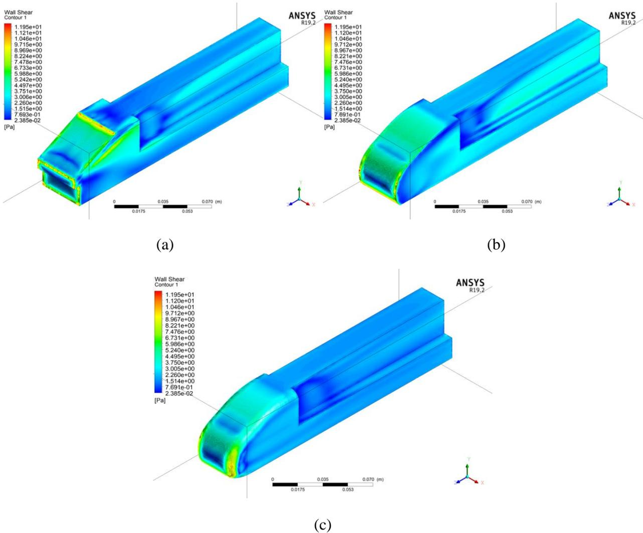
**Fig. 15** Shear Stress Contour in locomotive body in the Geometry Options (a) CC203; (b) 1; and (c) 2 at velocity 29 m/s. Seen, the shear stress is decreasing as the design change.
