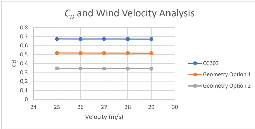
Fig. 11 Graph of Comparison of Changes in Wind Velocity to  $C_D$  Value in the three locomotive nose designs
