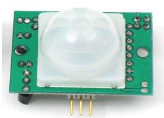
Figure 5. PIR Sensor (source : Kumar et al., 2015)
