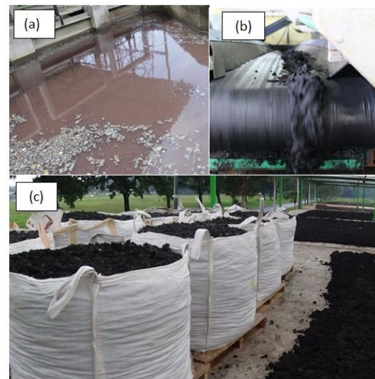
Figure 1. (a) The Industrial Wastewater ; (b) Mechanical separation of solid particles from wastewater; (c) Dried sludge
